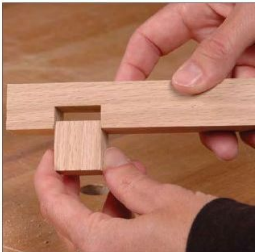
Figure 6—Use the gage block to test the width of the notches.
