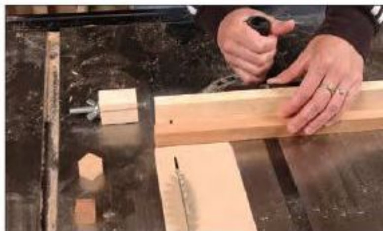
Figure 75—Cut the cubes to length using a fence stop and improvised holding clamp.
