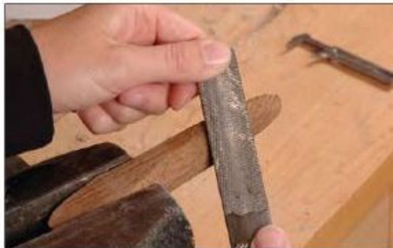
Figure 108—Shape the back of the Celt with files and rasps.
