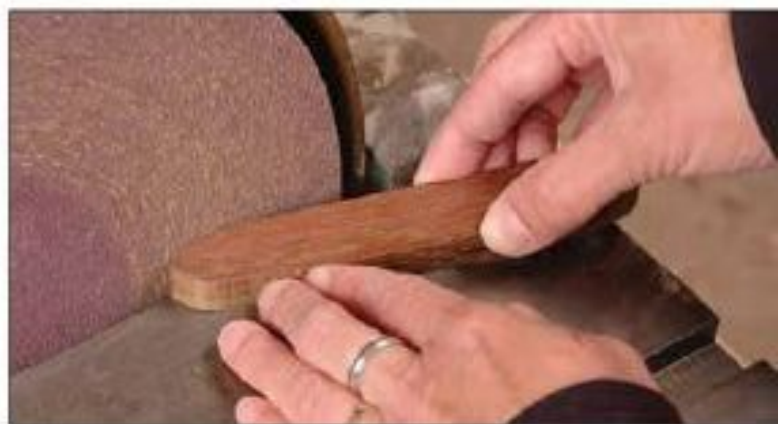
Figure 107—Clean up the contour of the blank using a disk sander.
