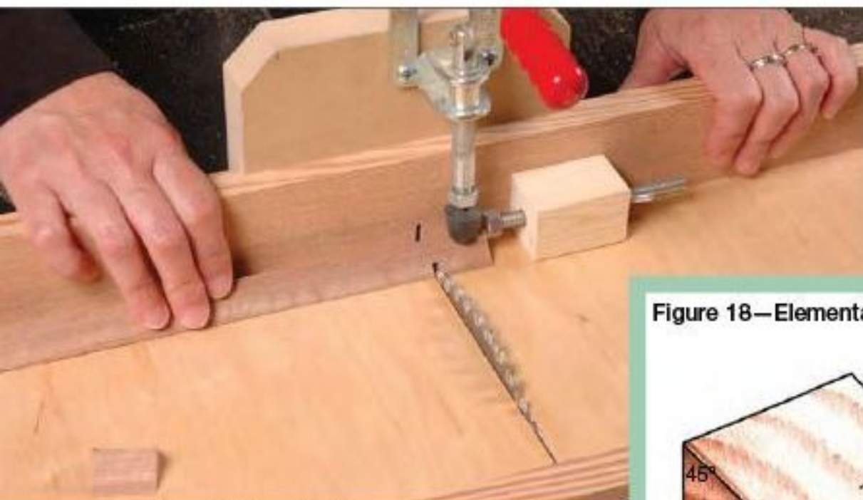
Figure 17—The prism pieces may be cut to length using a cross-cut box on the table saw. This box has a hold-down clamp and a micro-adjustable end stop. The stop block is glued to the jig base and fence.
