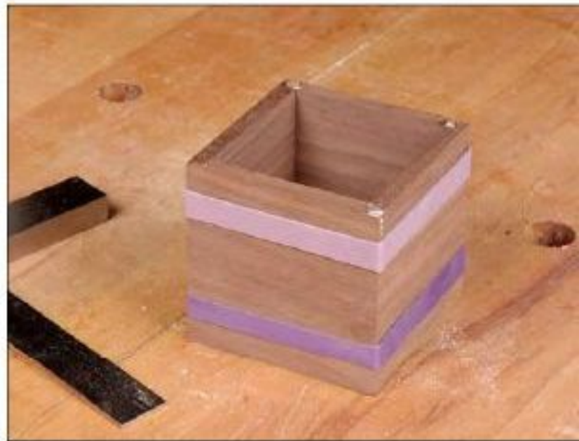
Figure 29—Use heavy rubber bands to clamp the assembled box while the glue dries.
