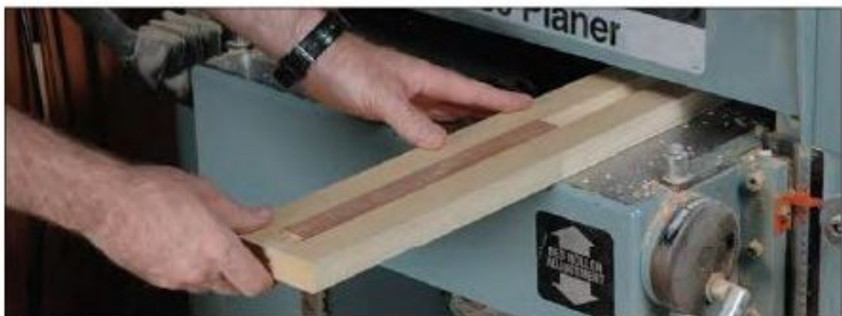
Figure 16— The long prismatic stick sits in the shop made cradle, ready to be pushed into the thickness planer.
