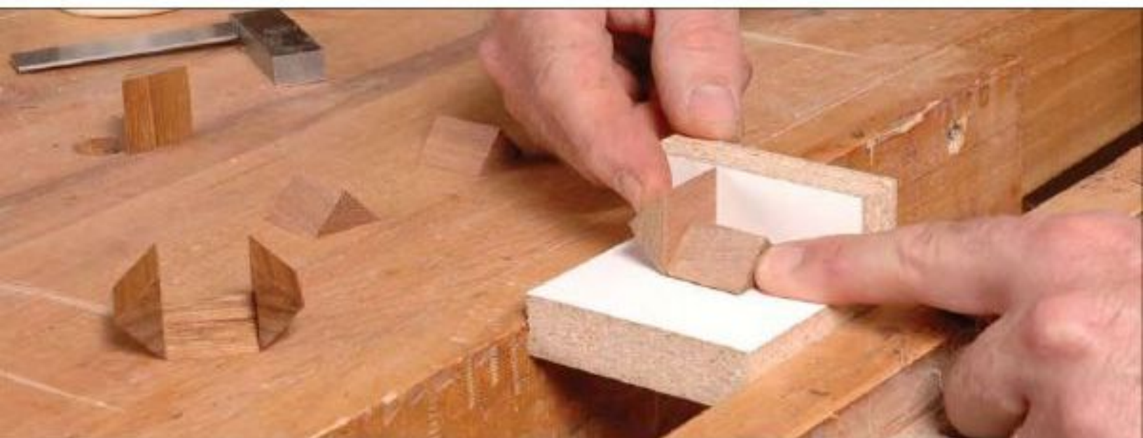
Figure 19—Make a simple fixture to help glue the puzzle elements together. Finger pressure is enough, until the glue grabs.
