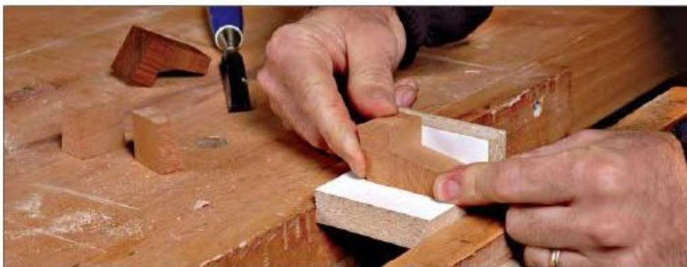
Figure 64—This simple fixture helps glue the puzzle elements together, by allowing you to push the pieces against the table and a stop.
