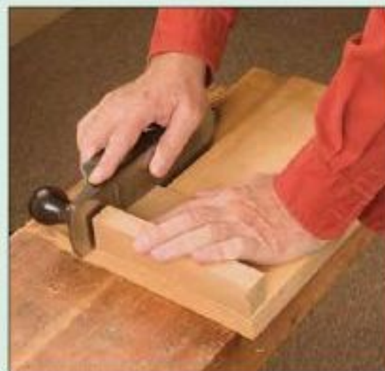
The bench hook is invaluable when dimensioning a small project part.
