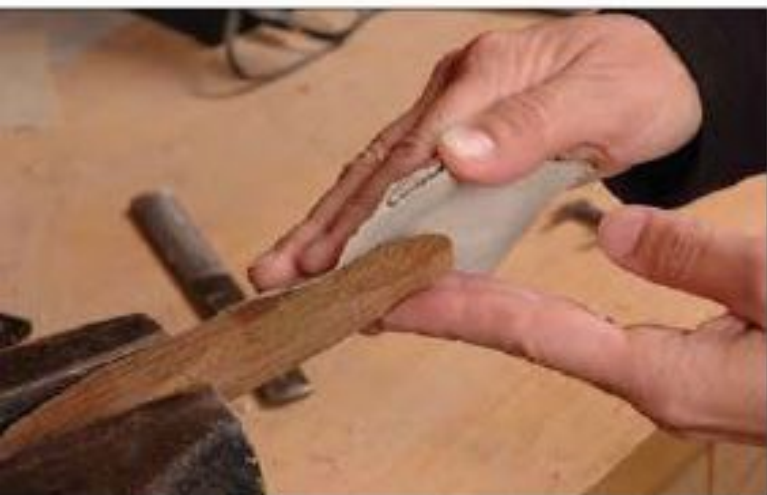
Figure 110 —Polish the surface by hand-sanding.
