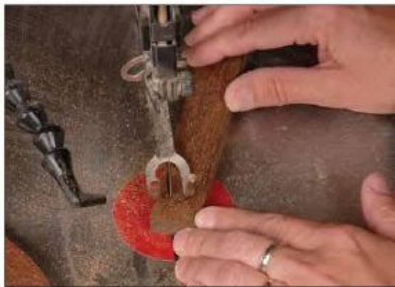
Figure 106—Cut the body of the Celt using a scroll saw or band saw.
