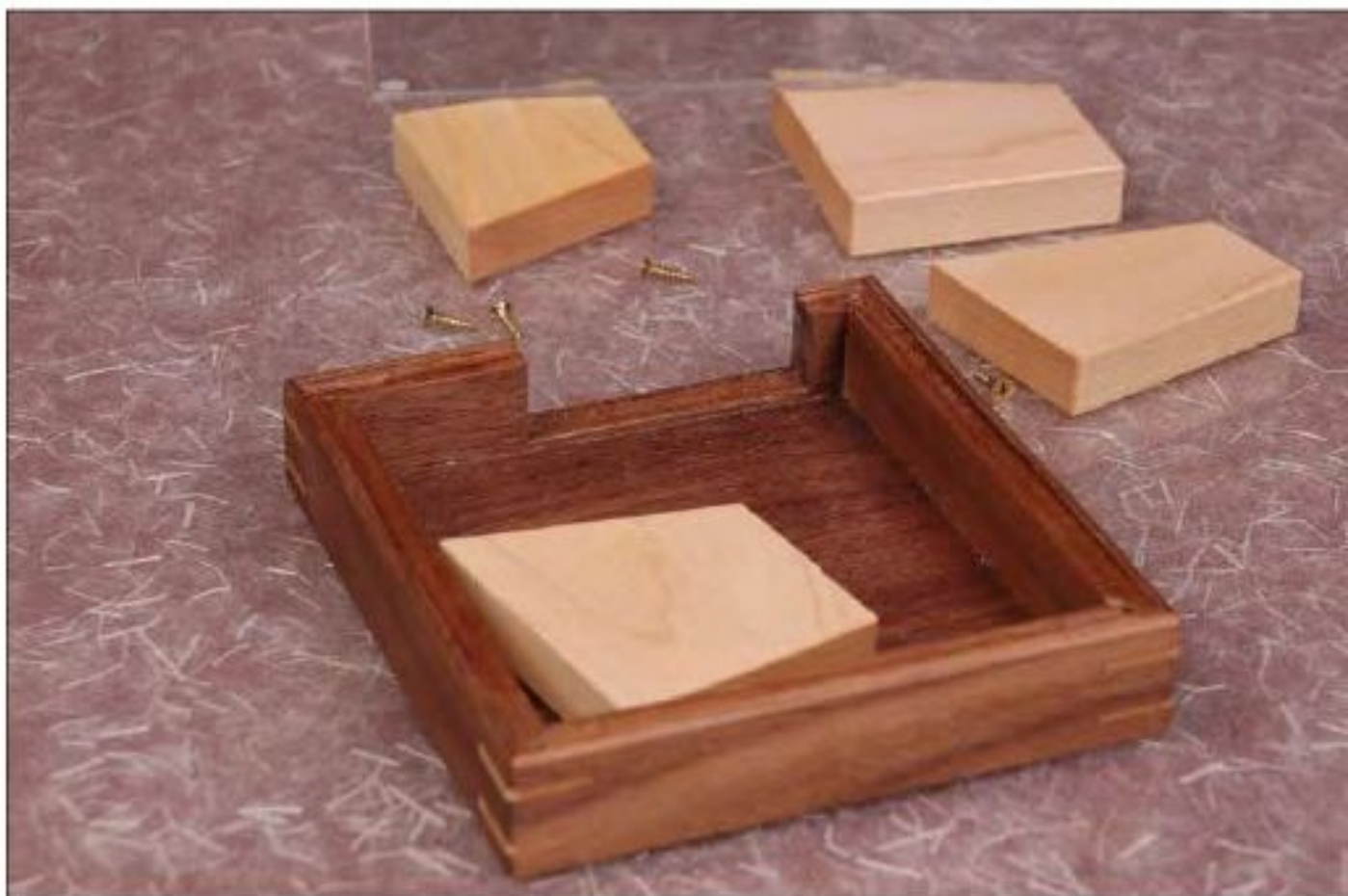
Figure 34—The small ledge at the bottom of the opening keeps the pieces inside the frame. However, it also means you have to turn the frame upside-down to remove pieces while you work on the solution.
