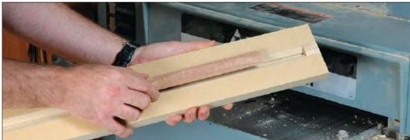
Figure 15— The shop-made cradle, with a stop at one end, is being used with a thickness planer.
