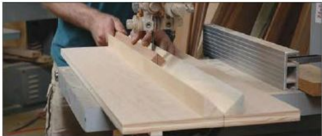
Figure 13—Saw the square stick down the middle on a diagonal to make two prismatic sticks. This photo shows the band saw set up; a table saw could also be used.
