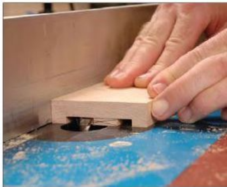
Figure 38—Use a straight bit in the router table to plow the tray cavity. The two side pieces complete the tray.
