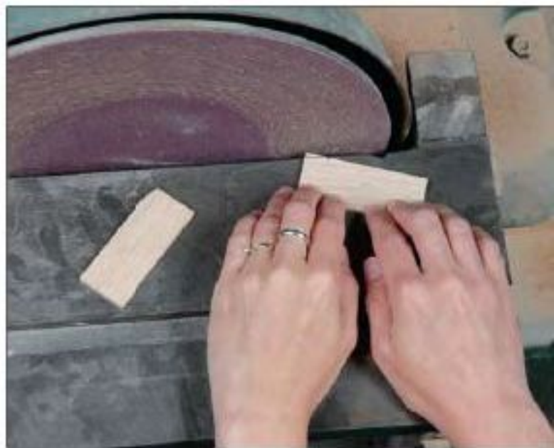
Figure 58—The disk sander, or a sharp chisel, will cut the small angle on the side liner pieces.
