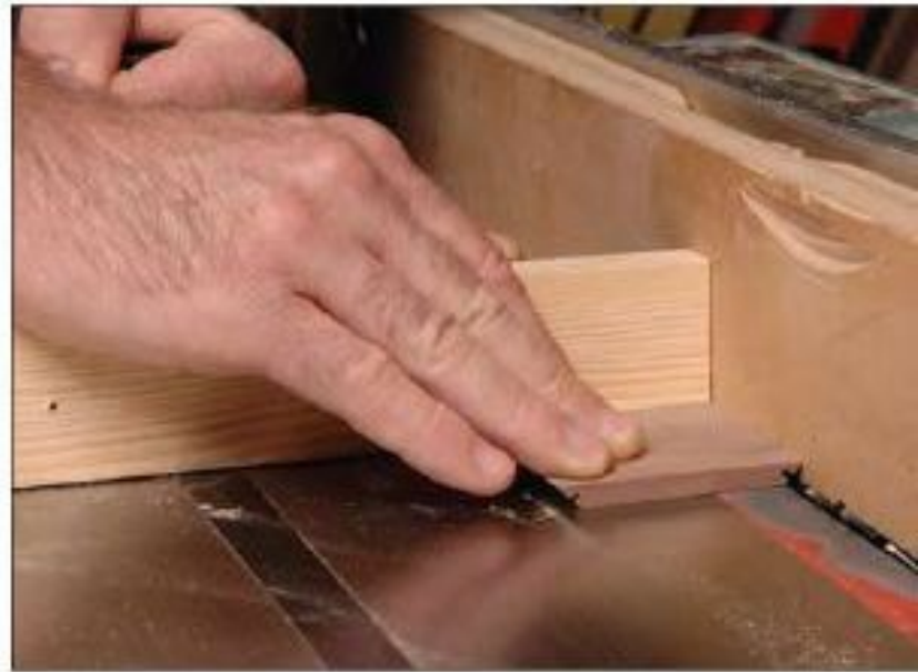
Figure 28—Cut the spline slot in the face of the 45-degree bevel on the table saw, using the miter guide and the rip fence.
