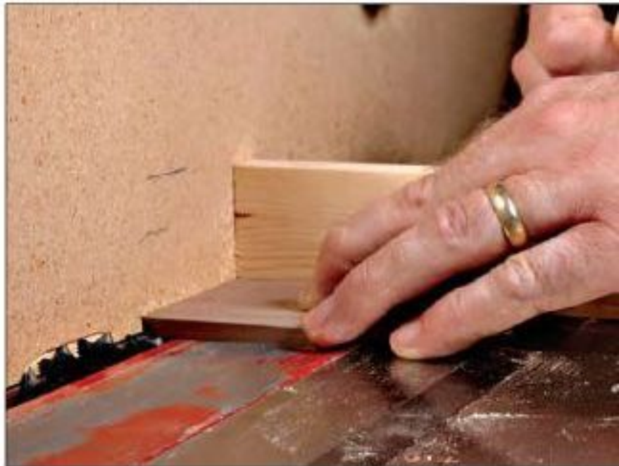
Figure 25—Miter the box sides on the table saw, with the blade set at 45 degrees and with a sacrificial piece of wood clamped to the fence, to minimize torn grain. Watch those fingers!
