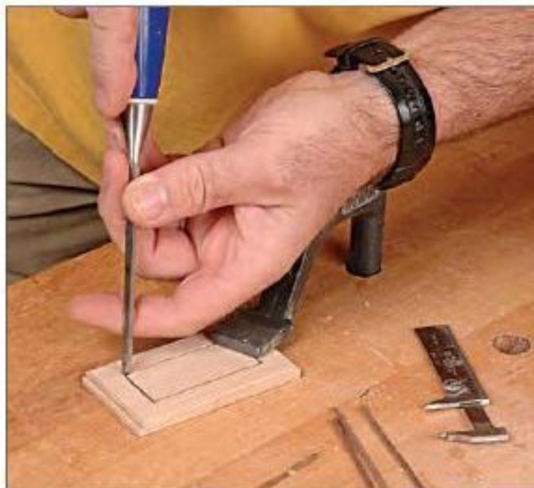
Figure 62—Rout the groove for the inlay in the box lid, and clean up the corners with a small sharp chisel.
