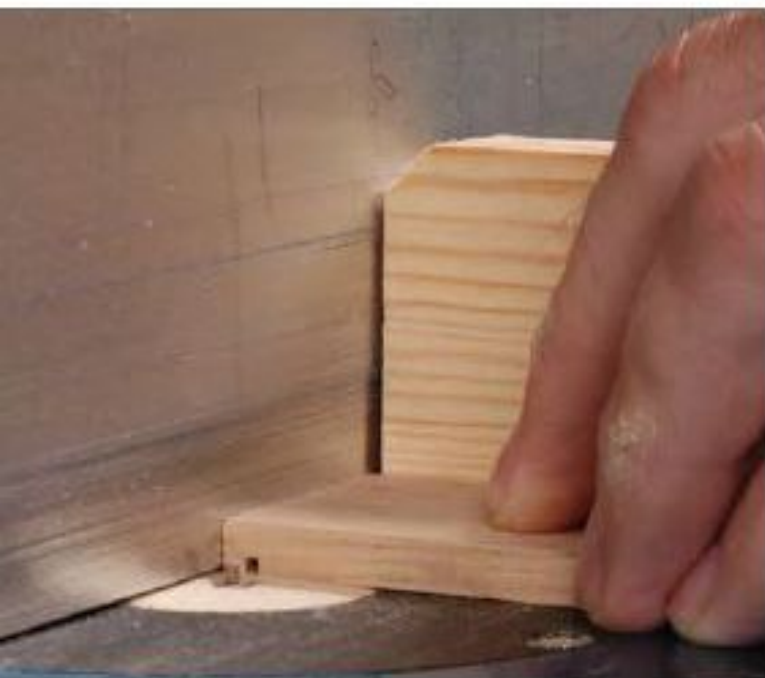
Figure 59 —Use the table mounted router with a \frac{1}{16} -inch bit to cut the dado for the corner joints of the box.
