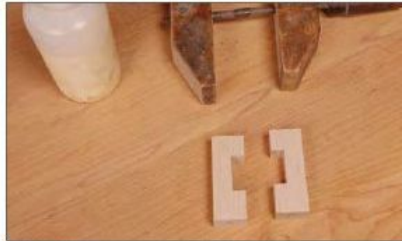
Figure 113—Both halves of each leg piece, already notched, are ready to be glued.
