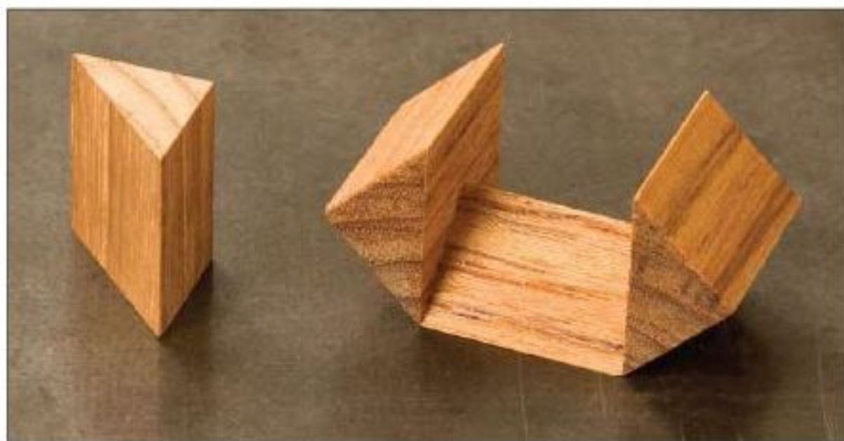
Figure 10—The six identical assemblies each consist of three prism-shaped pieces glued together.
